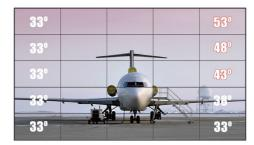
Without heat management, displays placed higher on a wall sustain more heat. However, NEC's advanced heat management ensures uniform heat dissipation.
