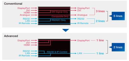
Just one cable each for video and control Only two cables required for setup . Up to 100 displays can be daisy chained
